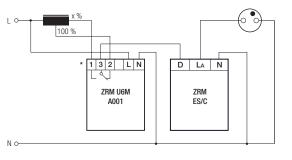
standby operation: pin 1 and 2 are connected 100 % operation: pin 2 and 3 are connected
