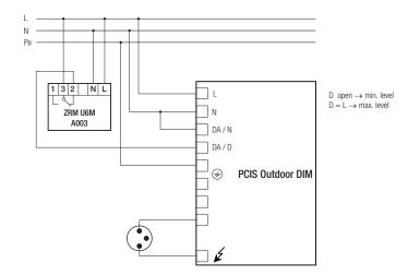
Circuit diagrams for power reduction in HID ECGs (e.g. PCS stepDIM or PCIS Outdoor DIM)
