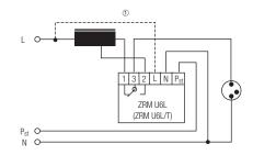
① wiring necessary at U6L/T because of the timer mode
