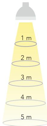
Note: Lux may be calculated by multiplying the Peak Intensity of the desired model number by the percentage in the tables above
