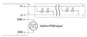
"DO NOT connect "DIM- to -V"
